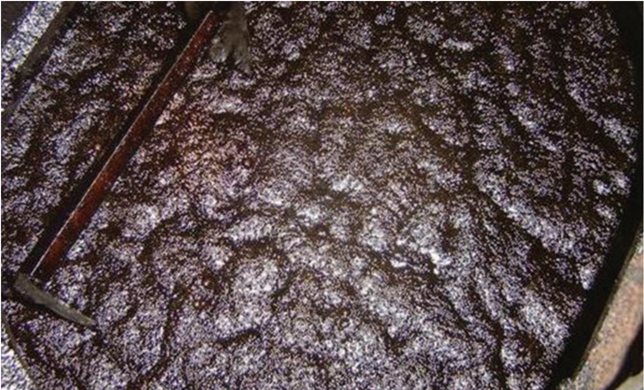
Fuel oil in a double bottom tank displaying frothing and foaming consistent with the cappuccino effect
