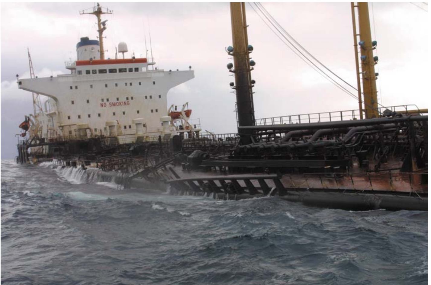
November 14 2002 - Damage to the starboard side (See enlarged views in Figure 9)
