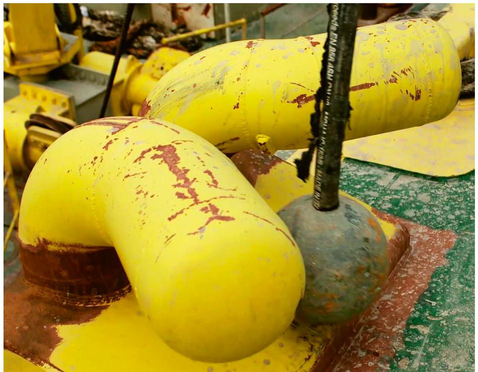
Figure 2. A V-shaped mooring bollard
