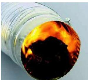
Don't forget about the hazards of lint-based dryer fires when you get home! The picture to your left is a typical home dryer duct. Cleaning out the ductwork at home periodically is just as important as the one on the ship!
