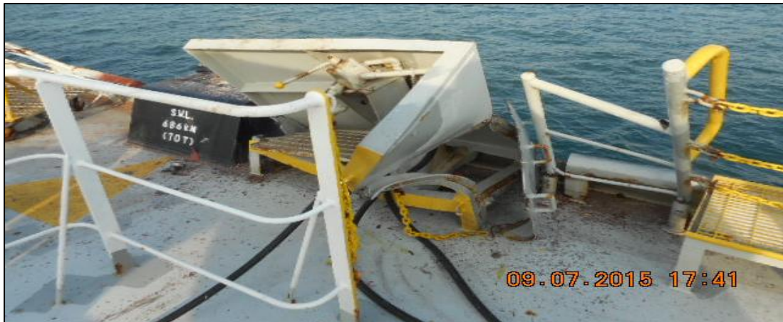
Figure 11: Damages to Brightoil Legend accommodation ladder, control station/panel damage and fairlead, which was torn off
