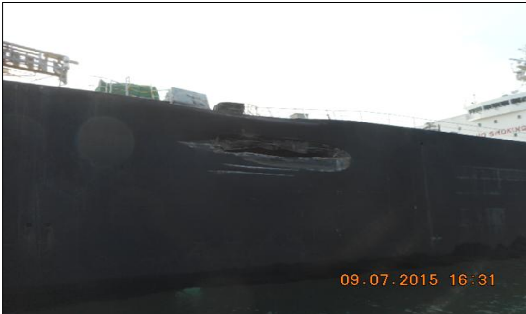
Figure 9: Damages to the Brightoil Legend side shell plating
