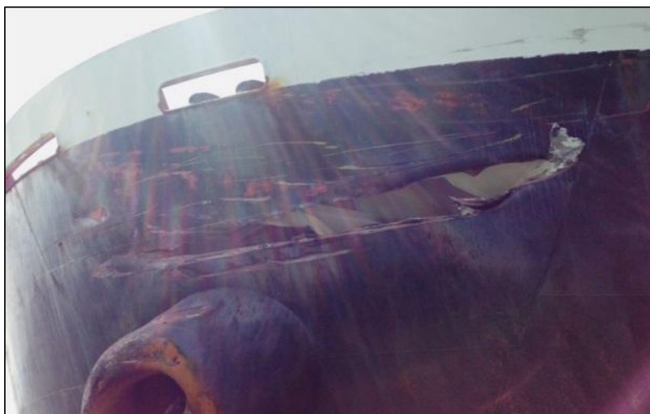
Figure 13: Damages to Capri's port bow shell plating
