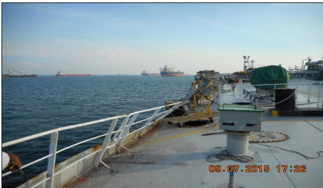
Figure 10: Damages to Brightoil Legend railing and fish plate
