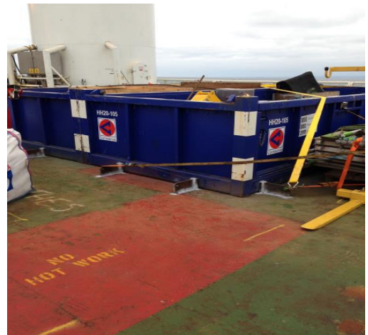
Clearly identified RED 'no hot-work' zones
