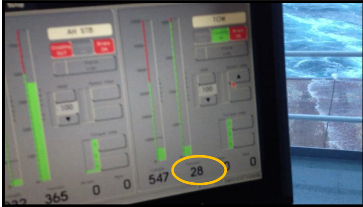
Figure 18: Screen capture from video showing tension reading of 28 tons on main tow drum. (Cell phone video screen capture provided by Mr. [REDACTED] AIVIQ Mate)
