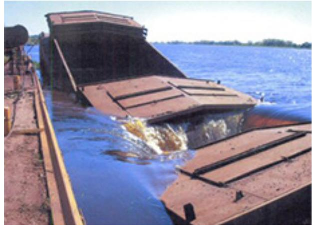
Fig. 1&2 Hull failure due to uneven distribution of cargo (sagging).
