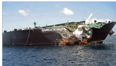
Damage to the Samco Europe following collision with MSC Prestige
