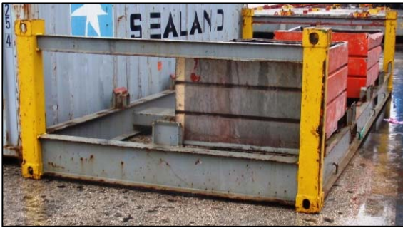
Figure 3: The frame used to hold the container lashing gear storage box used to lower the injured OS on the pilot boat
