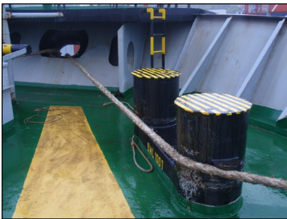
Figure 2: Purki 's forecastle showing the centre lead forward and starboard mooring bitts
