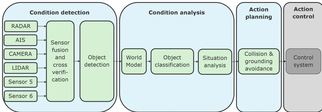
**Figure 1 Control of a function**
