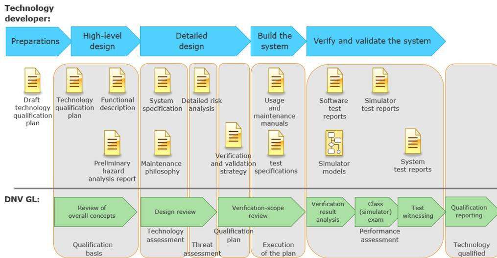
**Figure 12 Process interactions between the technology developer and DNV GL for technology qualification**
