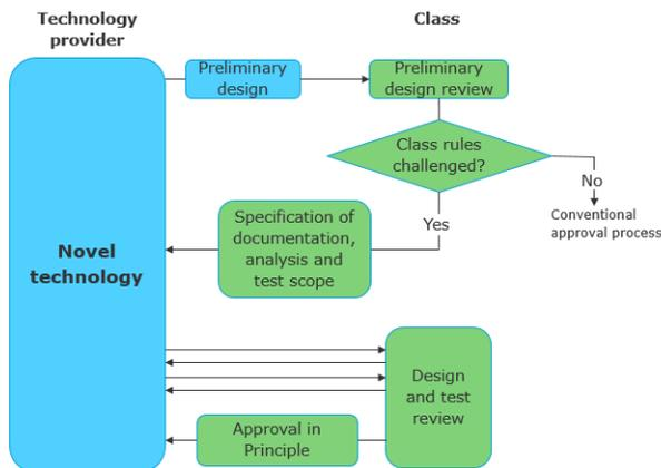
**Figure 8 Process for class approval of novel technology**
