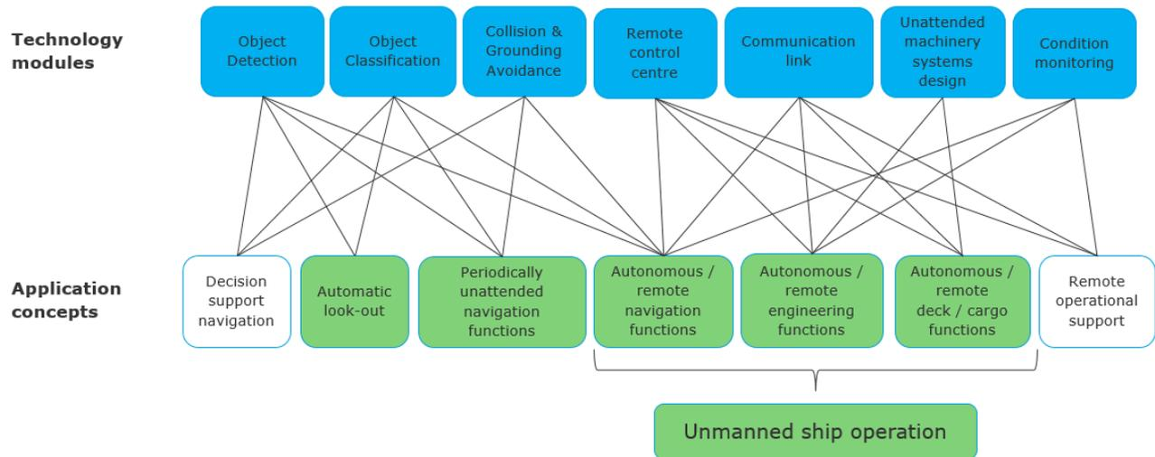
**Figure 2 Combinations of technology modules into new operational concepts**
