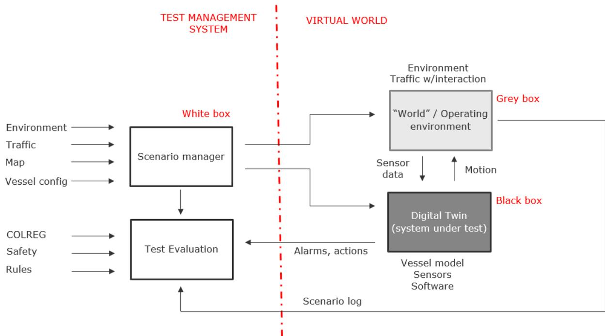
**Figure 1 Example of a simulator test setup for autoremoite navigation functions**
