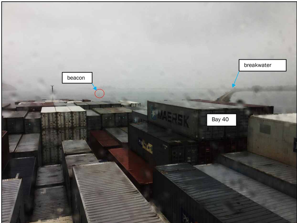
Figure 8 Example of an L-class ship where the beacon is about to be lost from view and the breakwater is obscured by the containers stowed six high (Photo courtesy of Port Otago)
