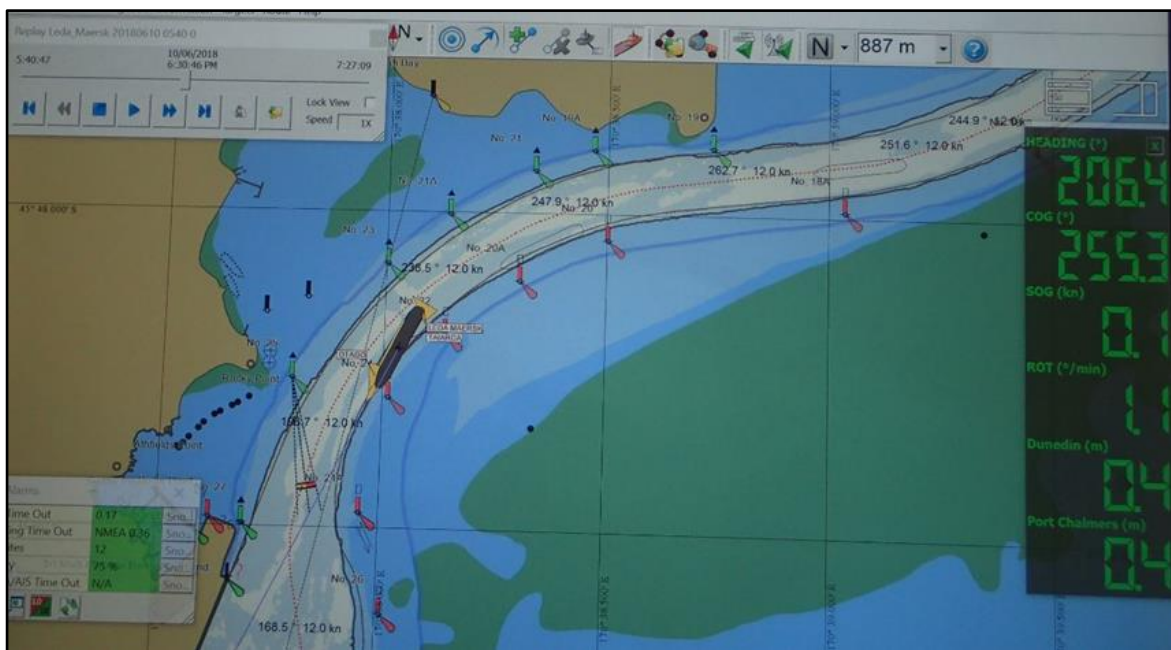
Figure 7 The Leda Maersk 's position displayed on the PPU at 1830, with past positions
