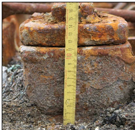
Figure 56: Height of container foot plus twist lock
