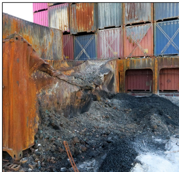
Figure 46: Slot 120782, unburnt pyrochar The contents spilled out when lifting.
