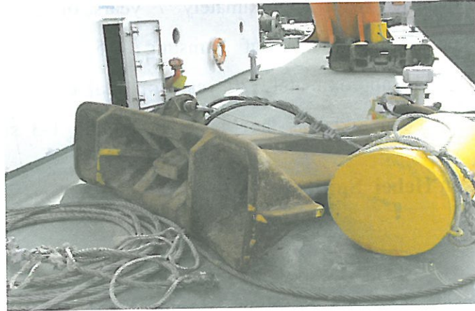
[Diagram 14] Positioning anchor and steel anchor buoy in yellow to indicate the location of Samsung No. 1's anchor
