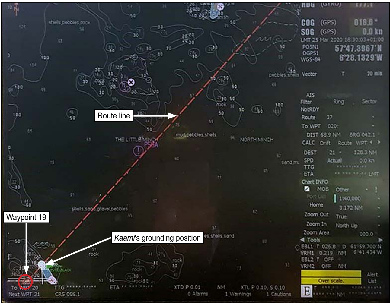
Figure 3: Kaami's starboard ECDIS showing waypoint 19
