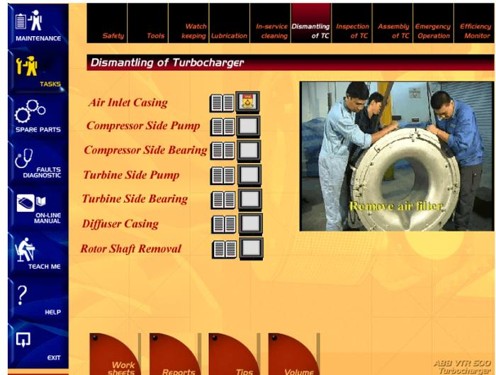
Fig.2 Turbocharger EPSS for VTR 500
