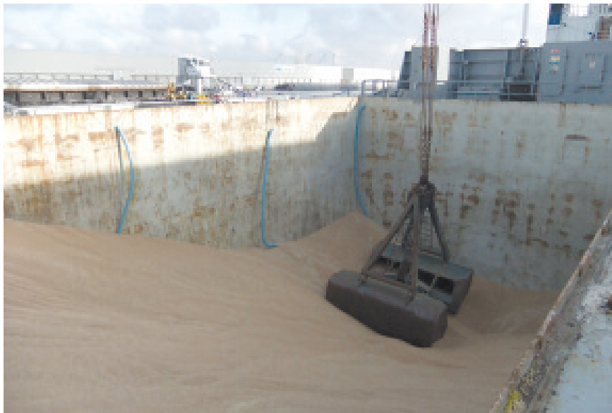
Grain being unloaded from cargo hold. Three out of six vertical plastic tubes can be seen. The aluminium phosphide tablets were placed into these tubes after loading. The tubes had small holes, but contact between cargo and tablets was probably insufficient so it took a full month for the fumigation to be completed in this case.
