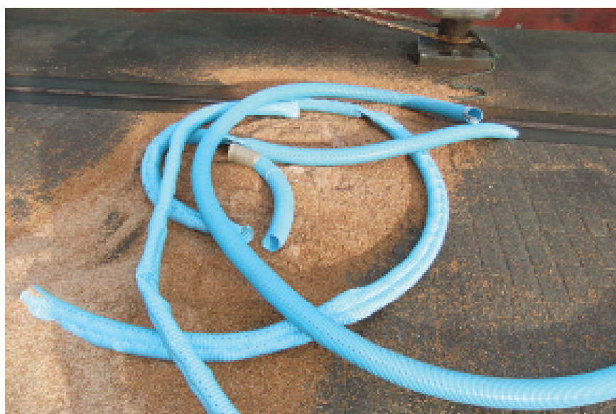
Plastic tubes used for aluminium phosphide tablets, pulled out after discharge of the cargo holds.
