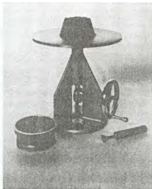
Figure 1.1.2 – Flow table and accessory apparatus
