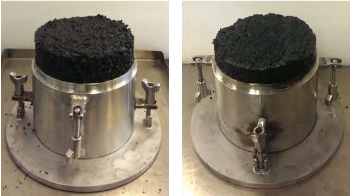
Figure 1.5.5.3.4.1 – Photographs showing valid tests for a partially saturated test portion (left) and a near fully saturated test portion (right)
