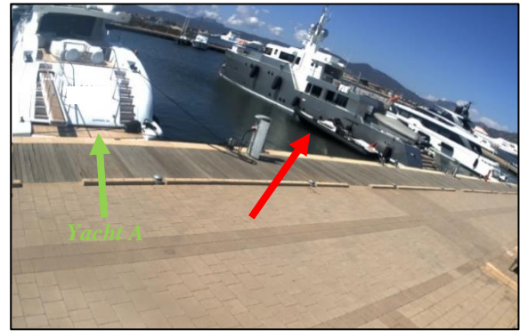
Figure 6: Still from the marina's CCTV footage, showing how Siempre was moored at Olbia (red arrow: Siempre , with her RIB moored to her port side)
