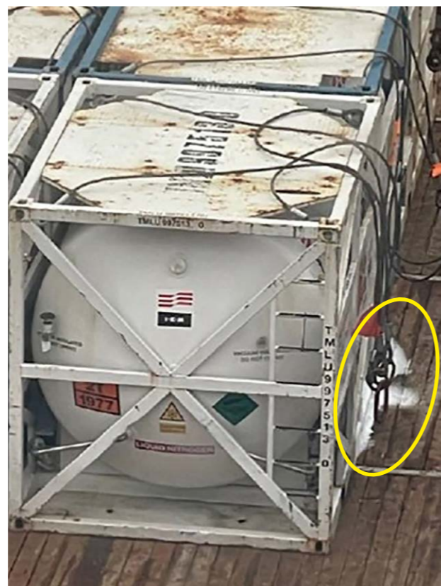
Figure 1: Icing of deck beneath nitrogen tank container
