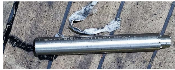
Figure 1: Damaged battery tube
