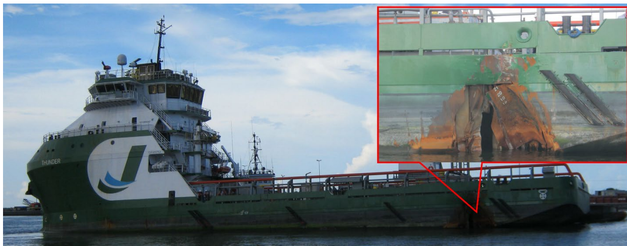
Figure 5. The Thunder being towed to a dock in Port Fourchon after the collision. The inset shows the damage to the aft port side of the vessel. (Source: Coast Guard)
