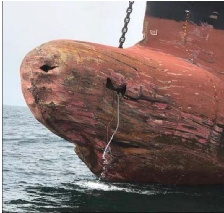
Figure 17: Holes and distortion in the bulbous bow plating
