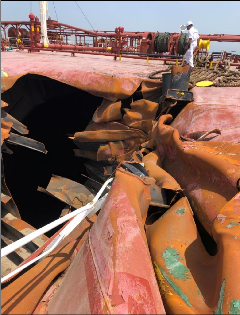
Figure 21: Damaged deck plating and fittings – as seen from the port side
