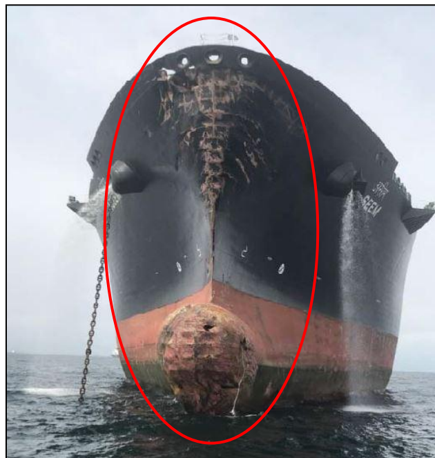
Figure 16: Damages sustained by Aseem , which was restricted to the region around the stem
