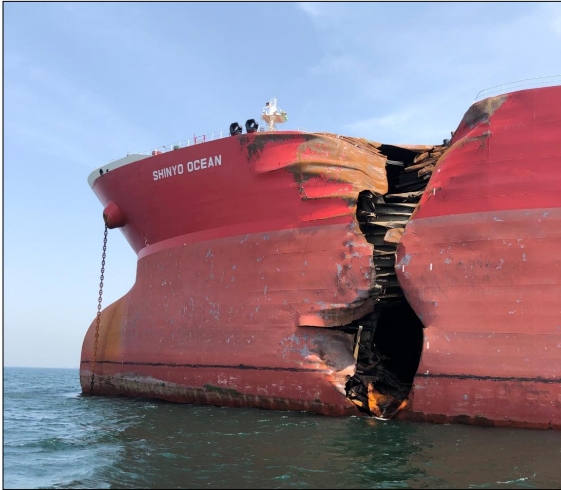
Figure 22: Penetrated hull plating (Source: Federal Transport Authority – Land and Maritime, U.A.E.)
