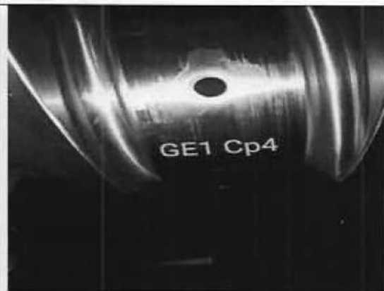
Crank pin found Wear ridge
