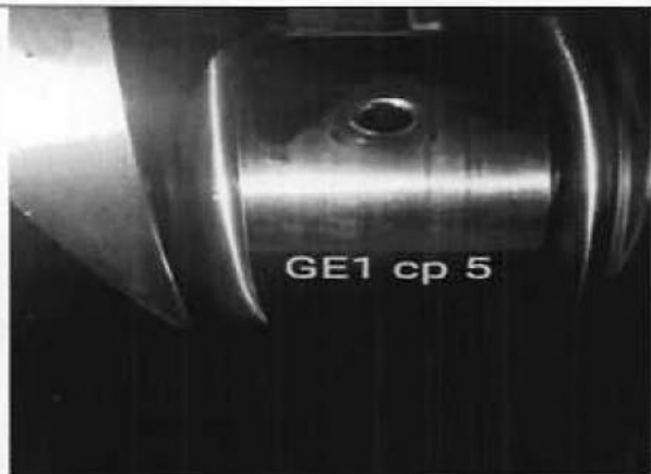
Crank pin found Wear ridge
