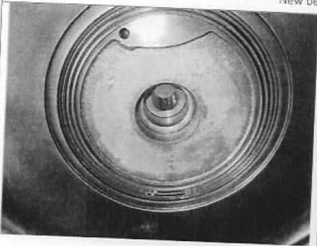
Bearing casing after cleaning
