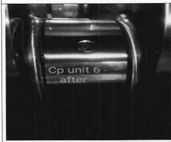
Crank pin after polished
