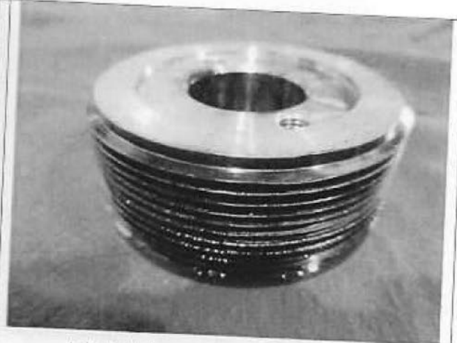
Labyrinth ring OD satisfactory – to reused
