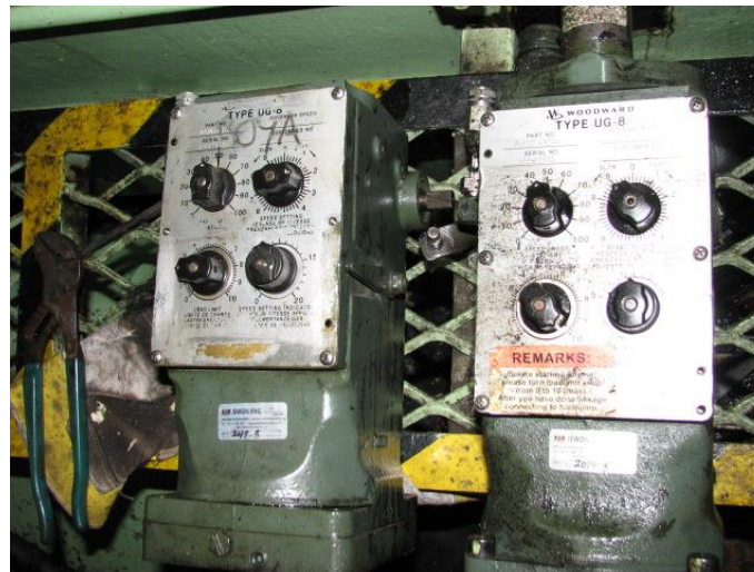
Figure 6. Governor C (right) was installed at the time of the casualty. Governor B (left) had been removed the day prior.
