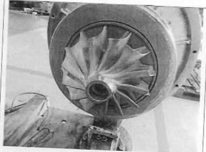
Assembling of rotor shaft to bearing casing
