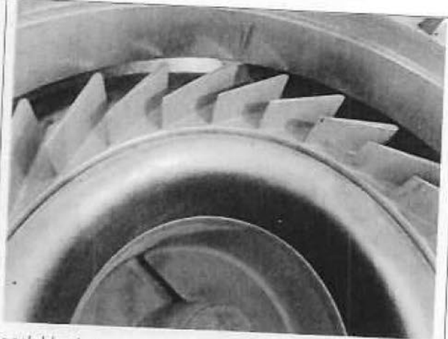
Nozzle ring after ash blasting
