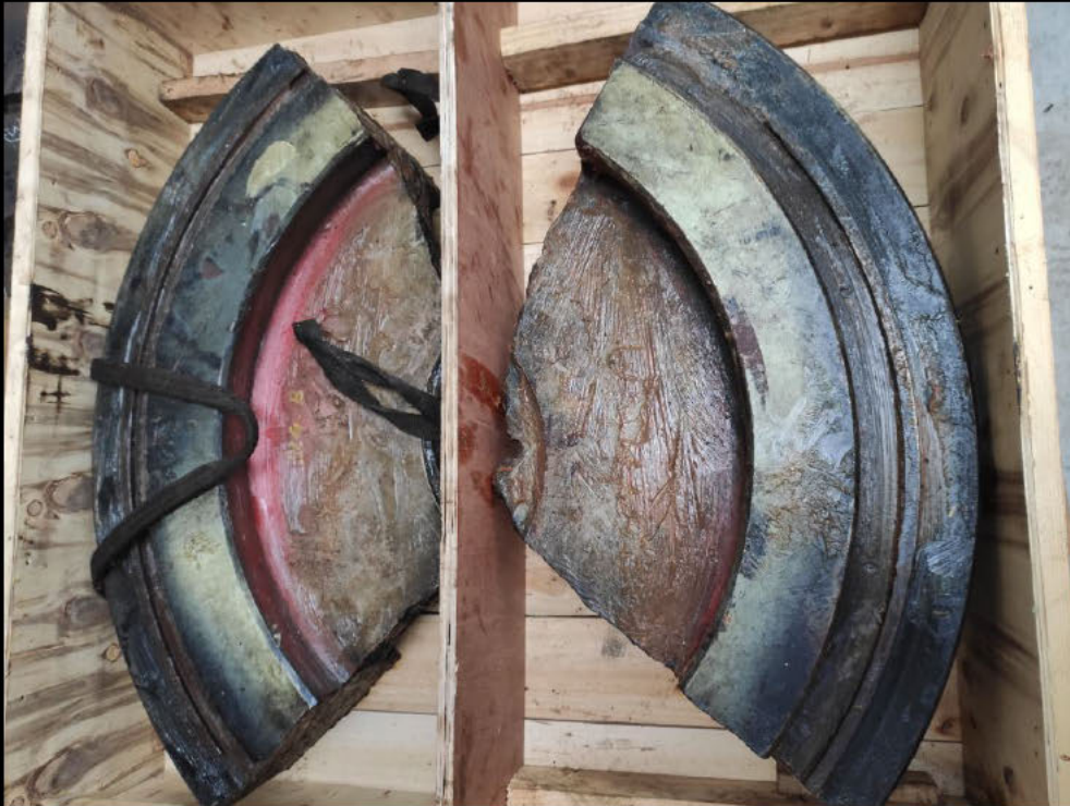
Figure 1 – Flywheel Fractured Sections
