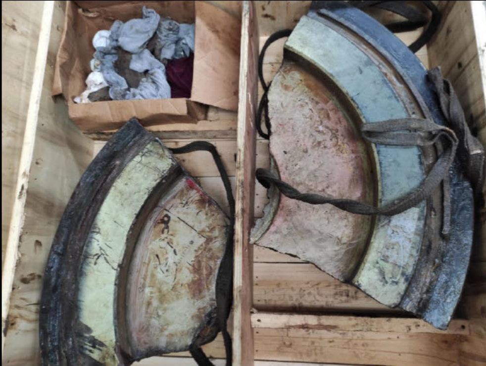
Figure 2 – Flywheel Fractured Sections
