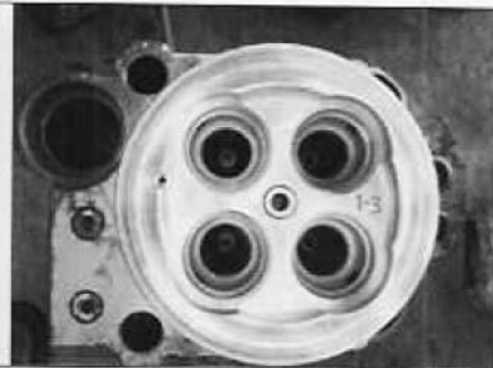
Valve seat pockets and combustion surface crack test
