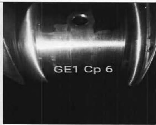
Crank pin found Wear ridge
