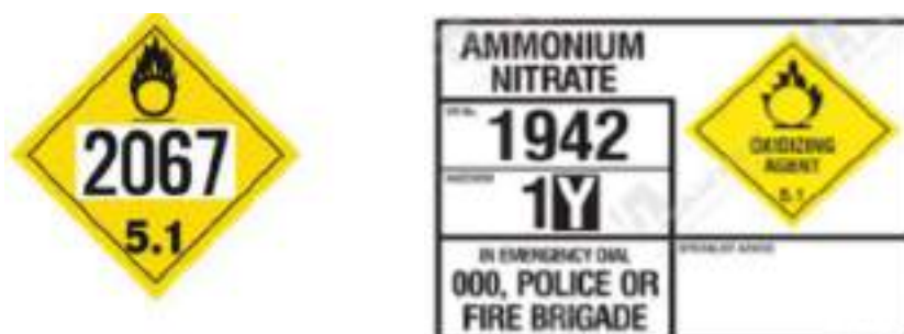
(Fig 1) Ammonium Nitrate Hazard Warning Labels
