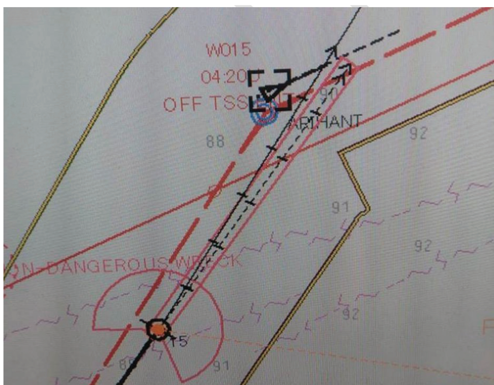
Figure 3: AIS Spoofing in the Strait of Hormuz. The acquired AIS echo only exists on the screen
